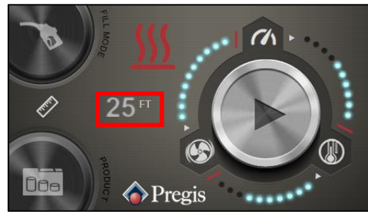
Figure 20. Both length and time per run can be adjusted by selecting the Run Time/Length icon.
