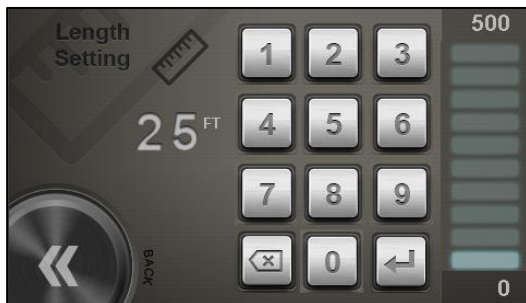
Figure 21. Length mode allows the user to select set length of pillow whenever the Start button is pressed.
