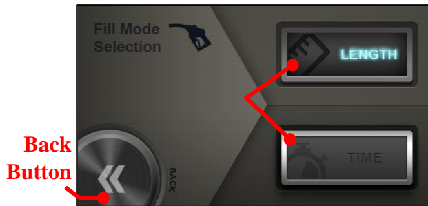
Figure 19. The Fill Mode Selection menu allows the user to toggle between length and time per run.
